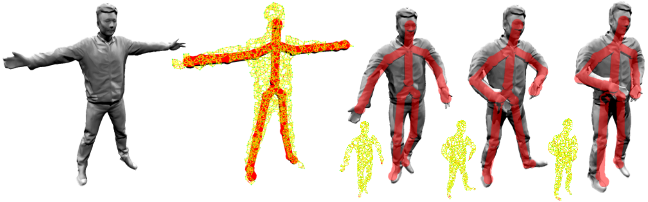
Figure 4: Animating a human avatar. User acquires a static 3D mesh of another human (left). The user can directly embed his skeleton inside the scanned mesh(center). Tracked skeletal motions produce realistic mesh deformations (right).
